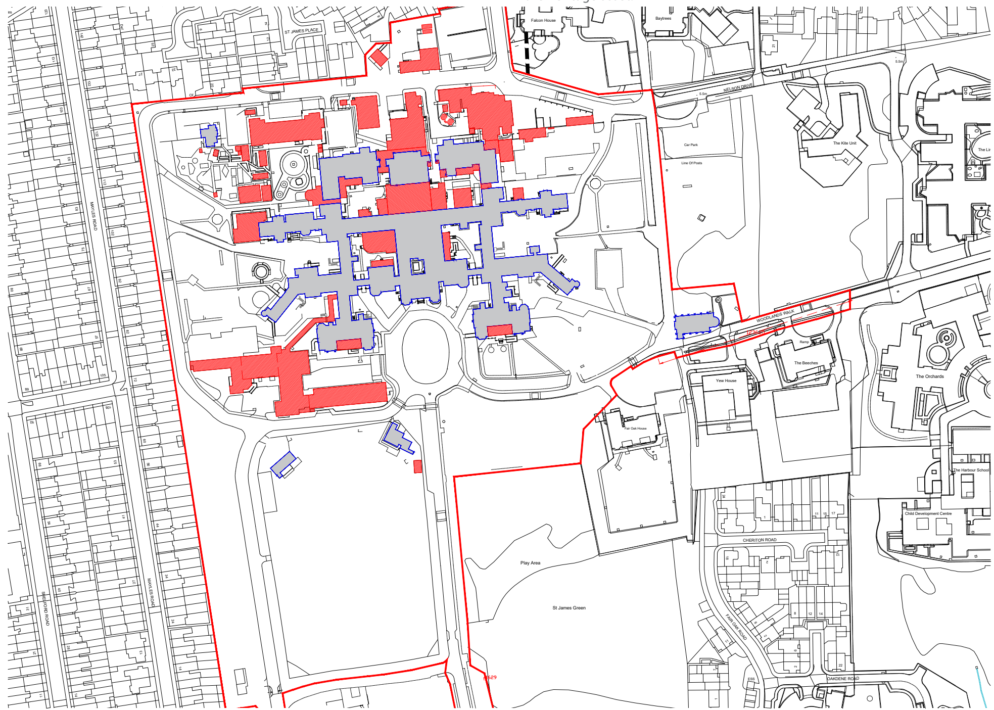
Image 40. Existing Site Plan showing the extent of Demolition proposed
